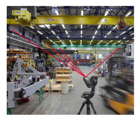
Measure two visible points on each wall
